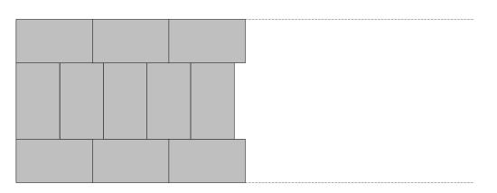
I lay the slabs lengthwise along the edges of the path and crosswise in the centre of the path, as shown in the diagram. When I have placed the final slabs in the pattern, I can, if necessary, make a single straight cut across the end of the path with my chainsaw, in order to leave an exactly rectangular paved area.
