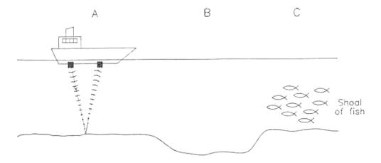
A monitor on the ship shows transmitted (T) pulses and any detected reflections <sup>®</sup>.
